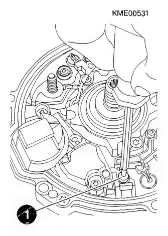
ASSEMBLING ALTERNATOR Assembling regulator Attach DF connection (1) to regulator. Use torque wrench. NOTE: Cable lug must be completely in recess of regulator (see arrow) to enable adhesive ring to be fitted. Tightening torque 1,0...1,4 Nm DF connection: comm. avail. Torque wrench: TORX T20: comm. avail.
